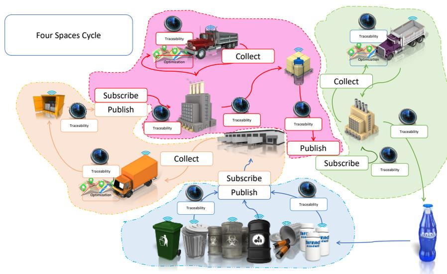
Specifically, the IPSE PARSIT architecture must allow: (1) management of messages from the LoraWan™ [\*] devices used, such as information regarding the filling of the waste oil container tank; (2) prediction of Best Date and Best Route for collecting oil; (3) management of a Marketplace for collected oil; (4) Tracking of collected waste using a Block Chain.
